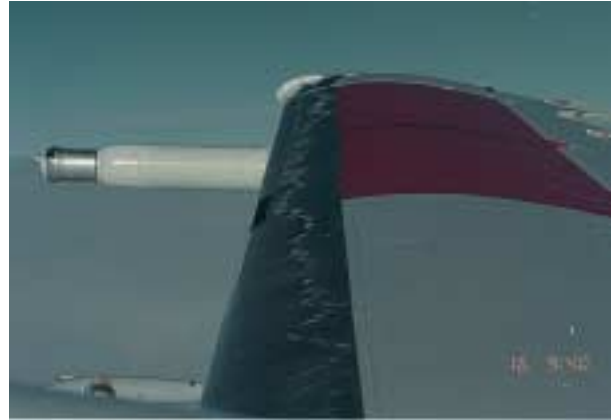
Figure 15: A photo of the Convair-580 showing runback ice close just aft of the heated leading edge of the wing for the severe icing episode of 16 February.
