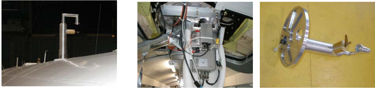
Figure 3. Photographs of the Nevzorov Probe mount and camera as used on the NRC-Convair-580 including from left to right: a) photo of roof of aircraft looking forward, b) camera mount inside cabin, and probe mount before installation on aircraft. The distance from the aircraft skin to the probe sensor is 38.4 cm, and the distance from the skin to the light is 49.5 cm.
